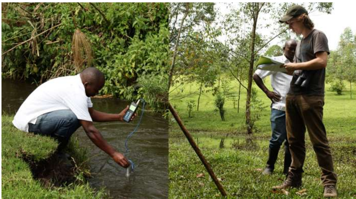
Figure 4. Recording stream velocity and completing the sampling site description form.
