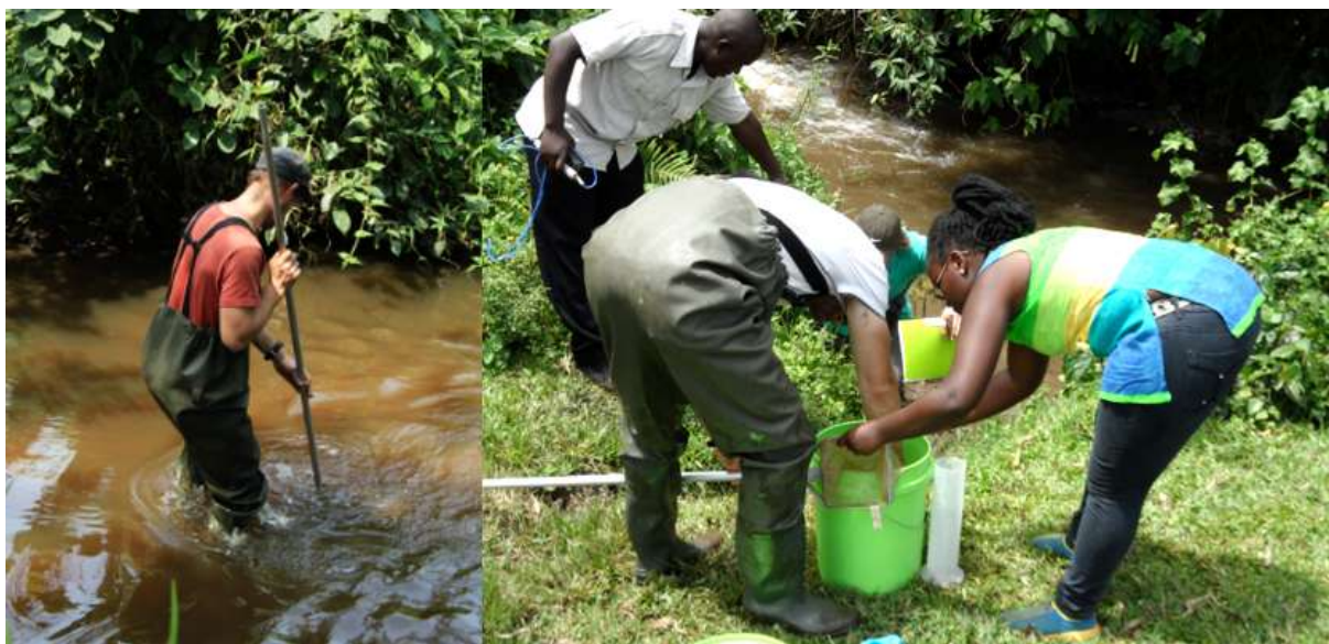
Figure 3. Macroinvertebrate collection by kick-sampling using a hand net (left), and transfer of the sample into buckets for transportation to the laboratory (right).
