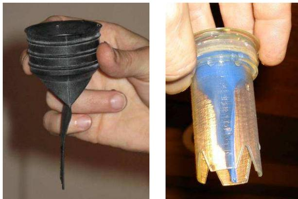
Figure 2. Two types of odour seals for waterless urinals: Left: flat rubber tube (Keramag Centaurus) and right: Transparent EcoSmellstop (ESS) unit showing the blue silicon curtain one-way valve inside (source: Addicom).
